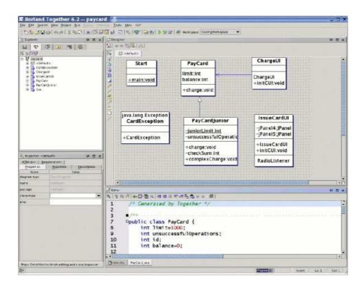
Figure 2: Class Structure of Tutorial Example
