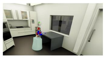
The humanoid robot ARMAR-III in a simulated environment for high-quality data augmentation. The input of the augmentation is an experienced episode. The output is a episode with modulated physical properties or different environments.
