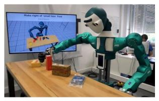
The humanoid robot ARMAR-6 predicts effects of pushing actions on objects in a table-top scene. Its prediction model has been learned offline and on simulation data. By incrementally learning from new experience, the robot could improve its prediction model.
