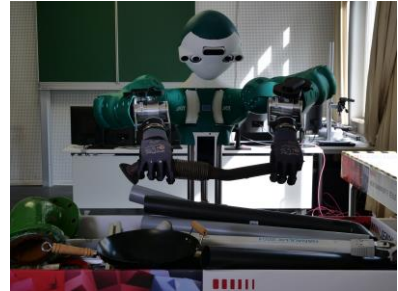
Fig. 1: The humanoid robot ARMAR-6 grasping unknown objects.
