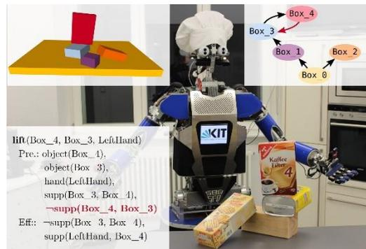
The humanoid robot ARMAR-III extracts objects and physically plausible support relations between them from its depth camera. Uncertain support relations can be used to predict undesired action effects.
