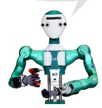
which actions may come next and which objects are required. Based on this understanding, the robot can offer assistance by asking whether it should perform an action or bring an object to the human to help. If the human confirms that they would appreciate help, the robot can finally execute the desired actions based on the task and action models.
