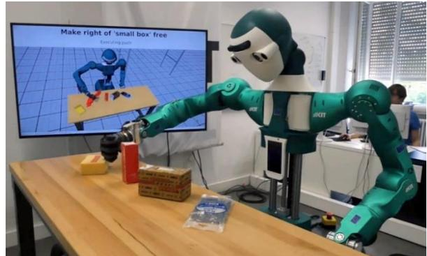
The humanoid robot ARMAR-6 predicts effects of pushing actions on objects in a table-top scene. Its prediction model has been learned offline and on simulation data. By incrementally learning from new experience, the robot could improve its prediction model.
